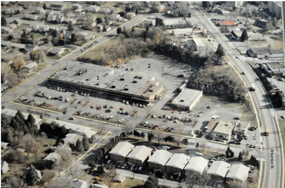
Figure 2: (a) Oblique aerial view of Rupp Quarry (center) showing mining at an approximate maximum depth of 70 feet. (b) Oblique aerial view of the Hamilton Square Shopping Center (#1) and Rupp Quarry (#2). By 1959, the quarry was backfilled to approximately 50 percent of its original total depth.
