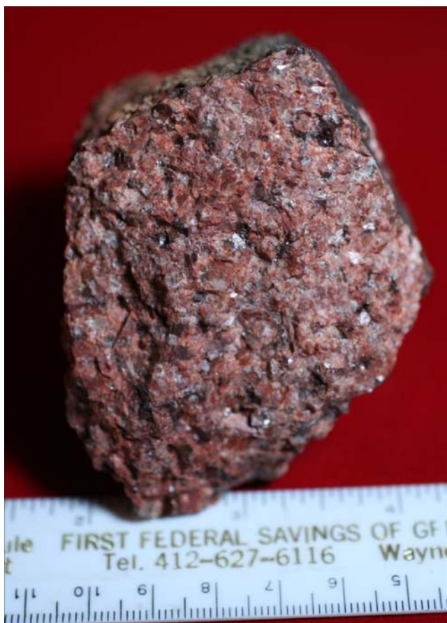
Figure 2. Coarse texture caused by slow cooling of magma beneath Earth's surface. Pikes Peak Granite. Minerals are quartz (pale gray), potassium feldspar (pinkish), and biotite (black). Plagioclase feldspar is also present. (Carnein photo and collection)
