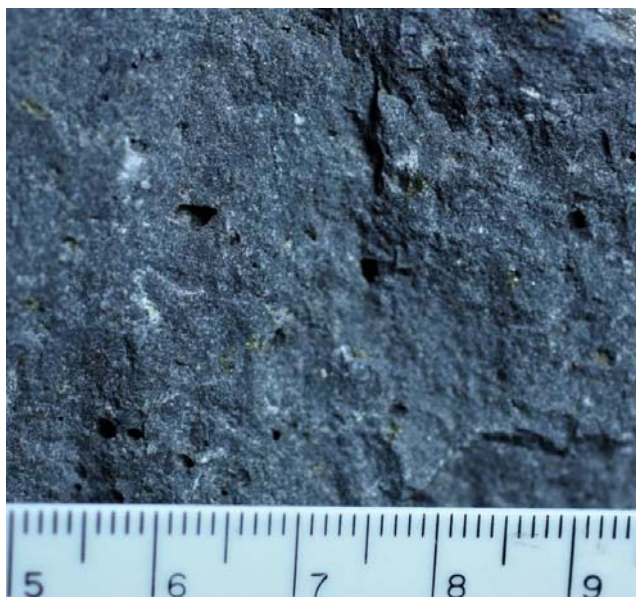
Figure 1. Volcanic rock (basalt), showing very fine grained texture due to rapid cooling from a melt. The rock consists mainly of plagioclase, pyroxene, and olivine. San Carlos Reservation, Arizona. (Carnein photo and collection)
